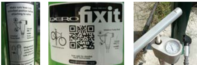
(Left and Center) Check out the information on the stations and on the pumps. QR codes will take you to "how-tos" on line. (Right) Open Eye pump with pressure gauge and dual head—one hole fits Schrader valves and one fits Presta Valves. The right one will fit tightly on your valve stem.
