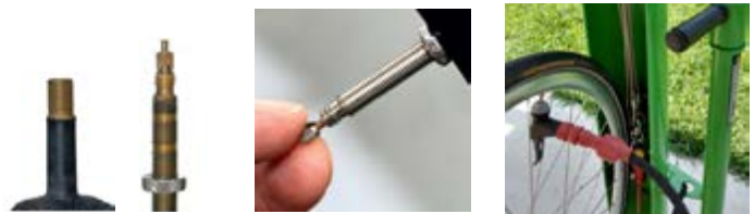
(Left) The wider valve is a Schrader valve, like the ones on car tires. The narrow valve is a Presta valve (yours may have a valve cap). (Center) If you have a Presta valve, you need to unscrew the top lock nut before you can add air. Press on the lock nut after it is unscrewed. You should hear air escaping if you have done it right. (Right) Once the bike pump is on the valve, you need to lock it on by pulling the lever up as shown here.
